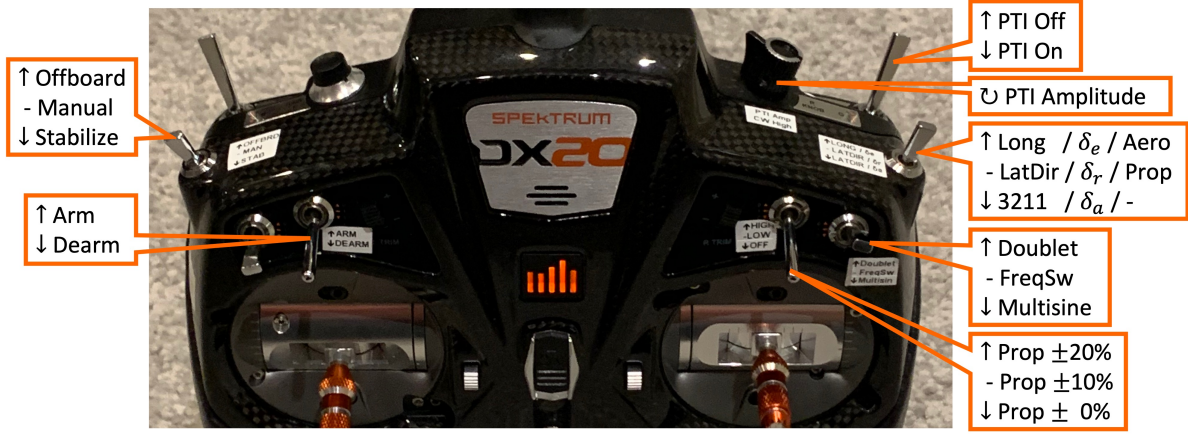
Fig. 3 Radio-controlled transmitter labeled for use with automated inputs and feedback control.
