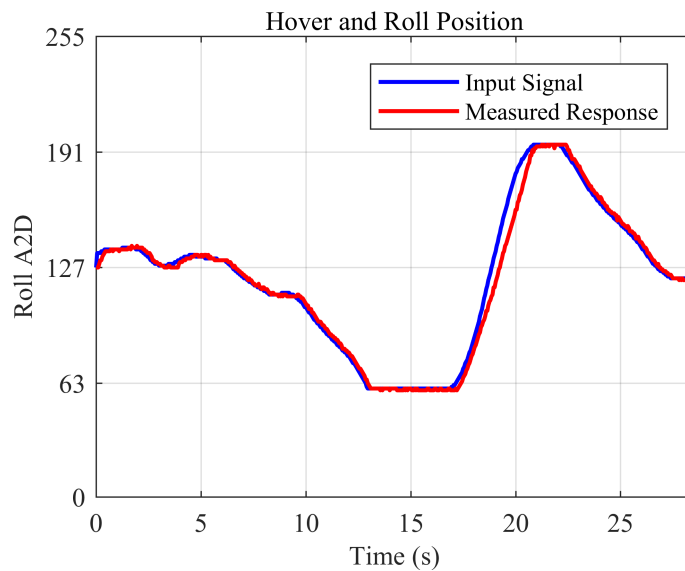
Figure 20. Flight data during hover to sideways flight
